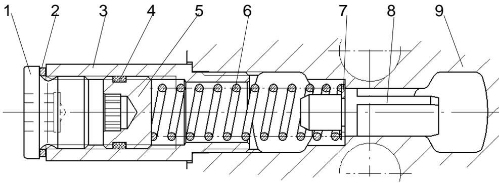
figure 6.1 – relief valves of pump types 101, 151 and 251
