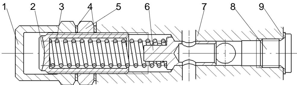
figure 6.2 - relief valves of pump types 51, 76, 351, 451 and 551
